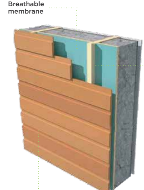
Horizontal boards Fastened at every intermediary support
